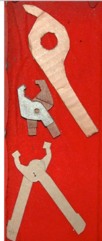
Leatherman® multi-tool prototypes created using wood (left) and cardboard (right).
