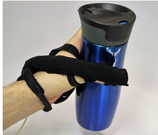
Figure 3: Example of a person wearing Pollex Grasp to complete an everyday task.
