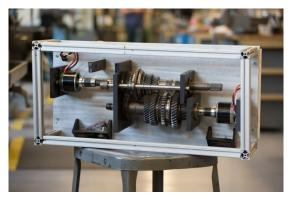
**The Solution:** A lightweight clutchless hybrid transmission that brings the best of the current hybrid architectures into one high performance, energy efficient vehicle. Dan is able to eliminate one of the largest sources of inefficiency in the transmission by removing the clutch, which can also reduce overall weight and transmission size.
